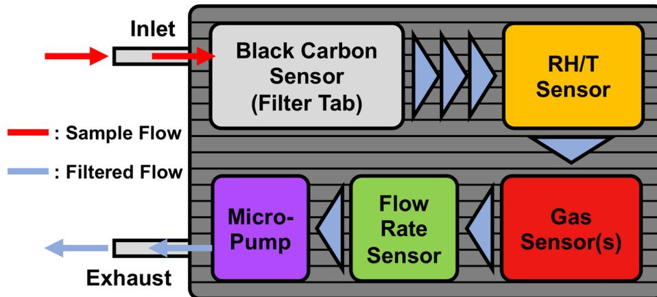
The ObservAir's micropump draws air through the fibrous aerosol filter. As particulate matter accumulates on the filter, the **aerosol absorption photometer** measures the rate of 880 nm light attenuation and calculates **black carbon** concentrations. Downstream, a **relative humidity and temperature (RH/T)** sensor monitors environmental conditions and **electrochemical cells** measure up to **two gaseous pollutants** simultaneously.
